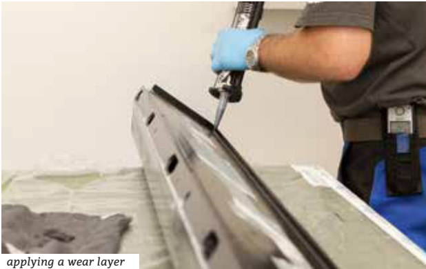
applying a wear layer
